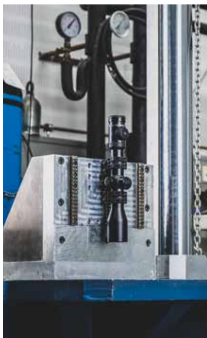
The V8 in the shock simulation test. Even after 800 shocks, the group remains unchanged.
